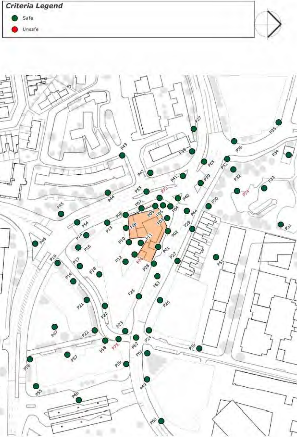
Figure 6c: Wind Tunnel Results – Proposed with Future Surrounds: Ground Level Plan, assessed against the safety criterion, (results shown with proposed vegetation)
