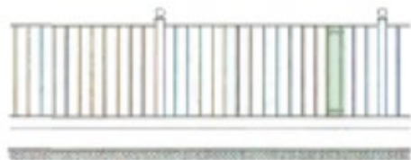
1:50 ELEVATION FROM ROAD SHOWING CLEAR POLYCARBONATE PANEL
