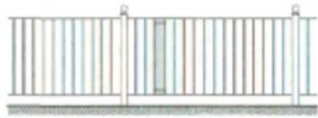
1:50 ELEVATION FROM FOOTPATH SHOWING CLEAR POLYCARBONATE PANEL
